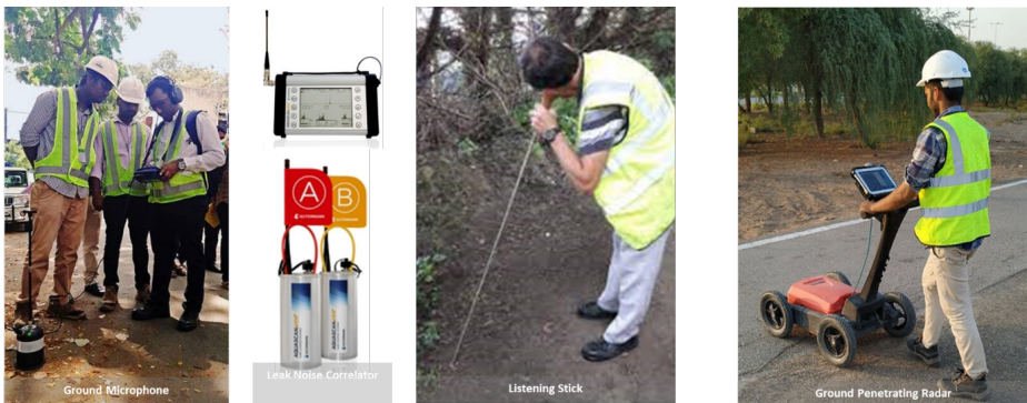
Figure 29: Leakage detection devices.
